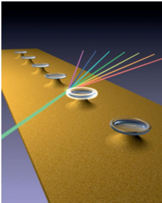
A microresonator breaks monochromatic light into a frequency comb.
