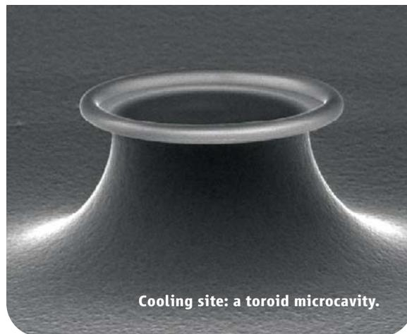
Cooling site: a toroid microcavity.
