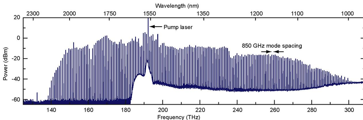
**Figure 2.** Octave-spanning spectrum generated from a continuous-wave pump laser in a microresonator.
